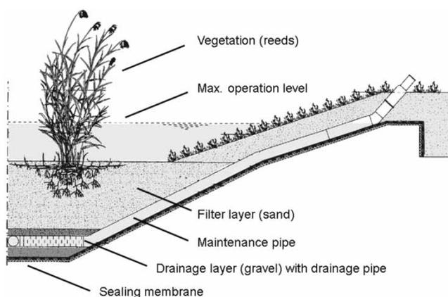
Figure 1 | Structure of a RSF, cross-section (MUNLV 2003).
